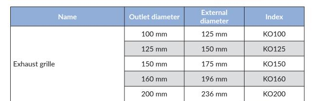
The airflow in the grille is adjustable, and in its back part there are steplessly adjusted holders for round channels.
